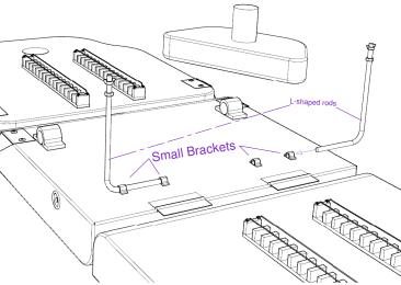
Slide the SHORT END of the L-shaped rods into the smaller brackets on the middle cushion. The long end of each rod should have one hex nut and one wing nut. For the next step. remove the WING nut but leave the HEX nut screwed down the rod toward the cushion.
