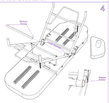
Now lin both sets of legs with the large brackets on the middle cushion. Take the leg anchoring bar and remove the small screws from each end and slide it through the aligned holes of both sets of legs and the large brackets. Once it is all the way through, it should stick out a little on both sides. Replace the screws into the ends of the anchoring bar to keep it from coming out of place.
