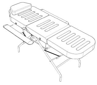
Insert the armrests into the holes with the zipper side facing down. The end with the zipper tab should face towards the foot of the bed.
